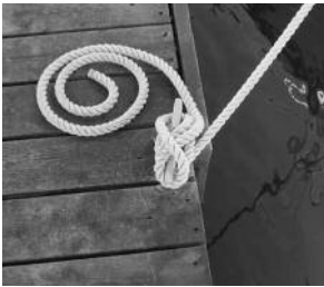
Above: a proper splice fitted well to the cleat.
