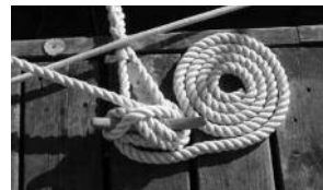
On the left is a great way to place permanent dock lines. The cleat is still relatively free for visitors to use.
